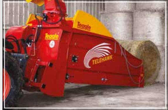
in the machine. Do not force the bale into the crossbeater. This will cause the machine to go into unblocking mode once the crossbeater is engaged. Place the chains around the rear of the bale. Cut and remove the strings. For easy removal of the strings place the bale on its side so that the strings are not in contact with the floor.
