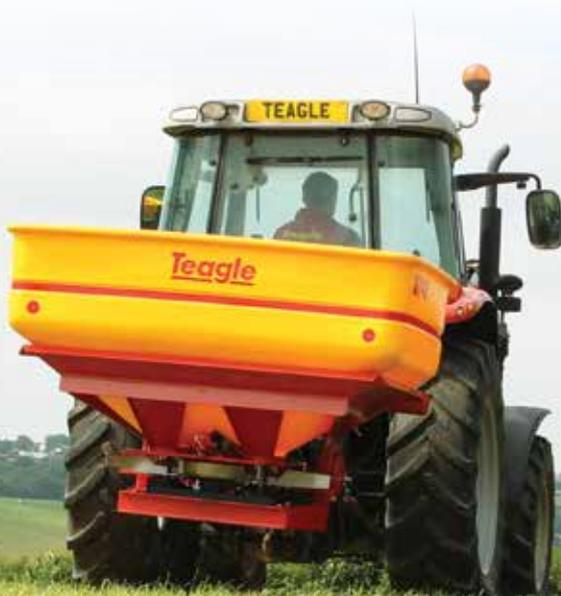
To spread headlands, the XT48 is fitted with a tilt system\* that concentrates the spread pattern in the area between the boundary and the first tramline, so that it accurately covers in 1 pass:
